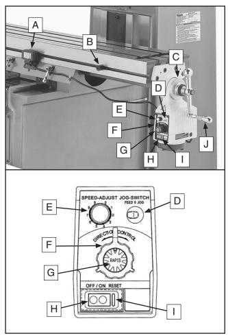
Figure 19. Power feed controls.
